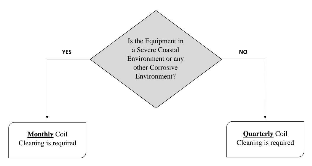
Severe Coastal Environment – Equipment is 3/4 of a mile off the coast, or less
