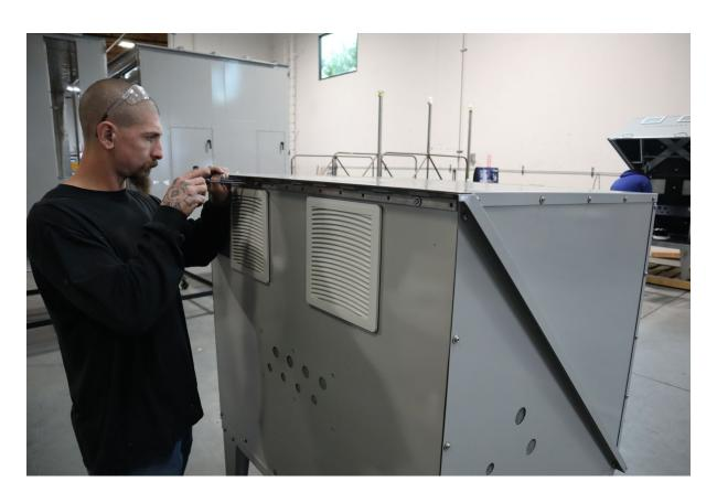
15. Install the hood-to-cabinet fasteners
