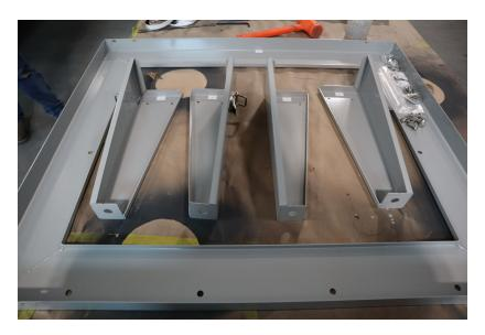
1. Unpackage contents and Assemble Front Stand Legs (1) and Rear Stand Legs (2 & 3) to the Stand Top (4)
