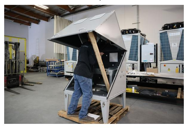
16. Prop the hood using a temporary brace as shown in the photos.
