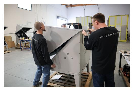
14. With assistance, lift the hood assembly onto the top of the cabinet, aligning the hinge and panel mounting locations.
