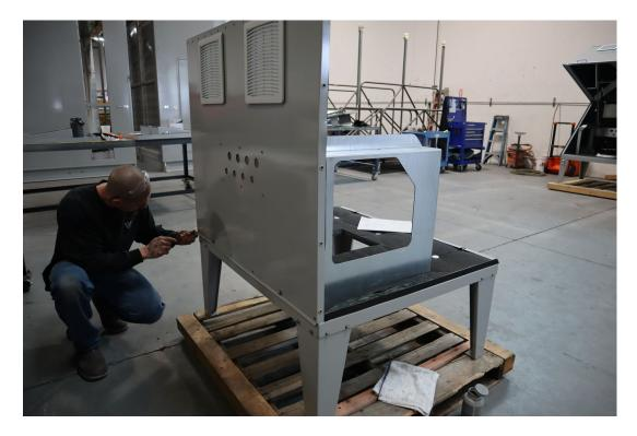
6. Screw in the bolts that hold the Rear Panel (9) and Bottom Panel (8) together
