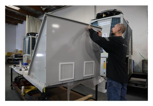
13. Install the external hood handles to the front edge of the hood
