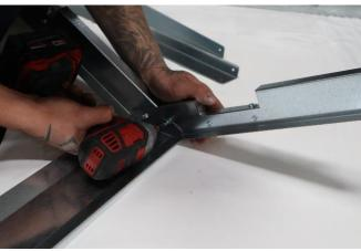
3. Overlap the Top Filter Racks (F1 + F2). The Left Filter Rack should be on top. Align the two holes with the Filter Rack Center (E). Screw together.
