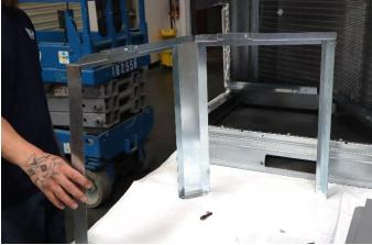
4. Attach the Filter Rack Sides (D) onto the inside of the assembled Top Filter Rack Part (F1 + E+F2)
